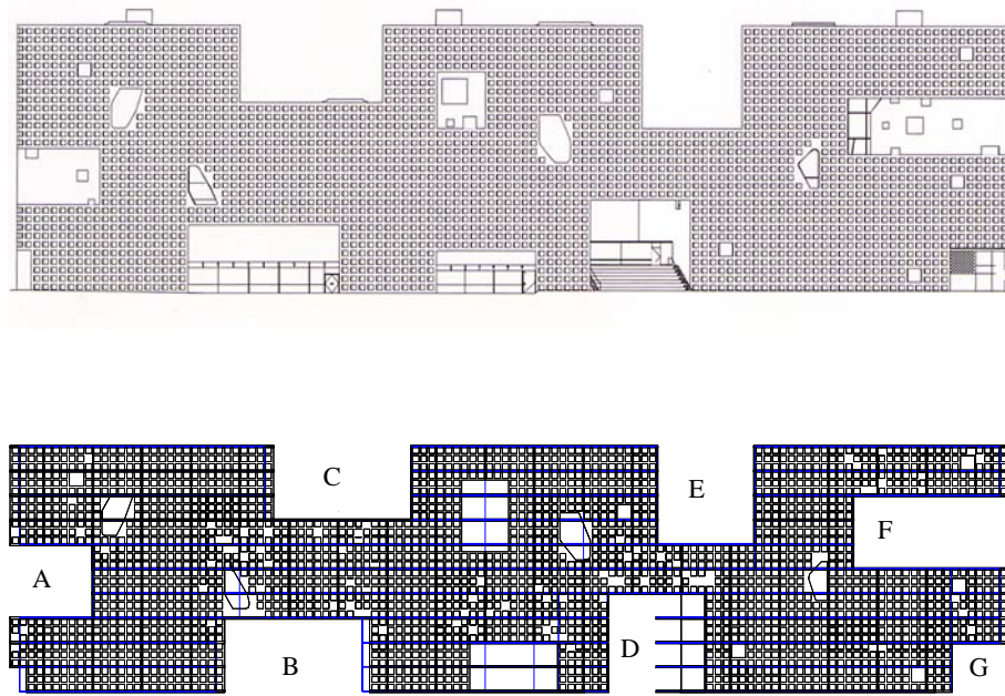
Figure 27. In the implementation of the building many of the large scale recesses of the building were blocked by spaces (up). A derived representation of the same view according to the conceptual rules appears below.
